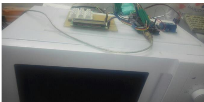
Figure 6. Modified Microwave from outside
