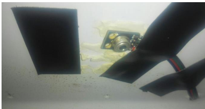
Figure 5. Temperature sensor mounted inside microwave oven
